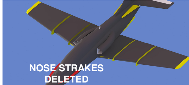
Fig 2. AC Configuration with Stall Fixes
